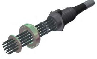
2. Thread the jack onto the strands. A suitable lifting device should support the weight of the jack.
